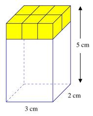
Since the prism has a height of 5 cm, there are five layers which are each one-centimeter thick. Since each layer contains six cubic units, the volume V of the prism is V = 6(5) = 30 cm<sup>3</sup>.
