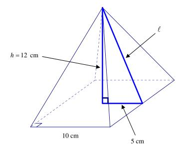
Since the altitude of the triangle intersects the center of the base, we know that the horizontal leg of the right triangle is 5 cm (half of the 10 cm side of the square base). We then use the Pythagorean Theorem to find  $\ell$ :
