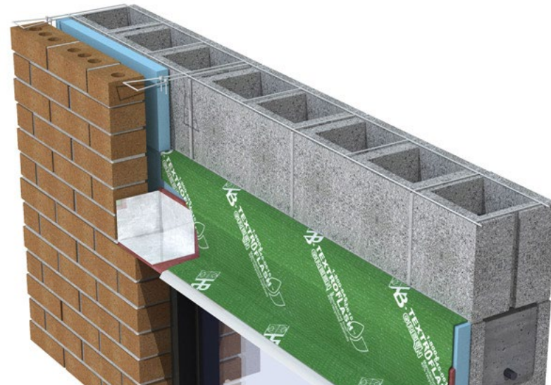
Diagram of properly installed end dams. (Image courtesy of h-b.com)
